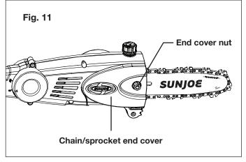
**NOTE:** If the chain is too tight, it will not rotate. Loosen the end cover nut slightly and turn the chain tensioner 1/4 turn counterclockwise. Lift the tip of the guide bar up and retighten the end cover nut. Ensure that the chain can be rotated by hand without binding.
