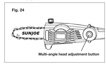
3. Adjust the head to the desired position (Fig. 25).
