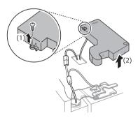
Detach the wire harness (1). Unscrew the ground wire (3) on the InstaView model only.
