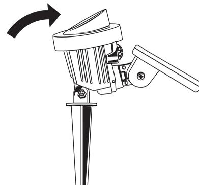
5. Push stake into ground and aim light at desired location.
