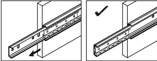
1. Pull out slide. Slide bearings forward.
