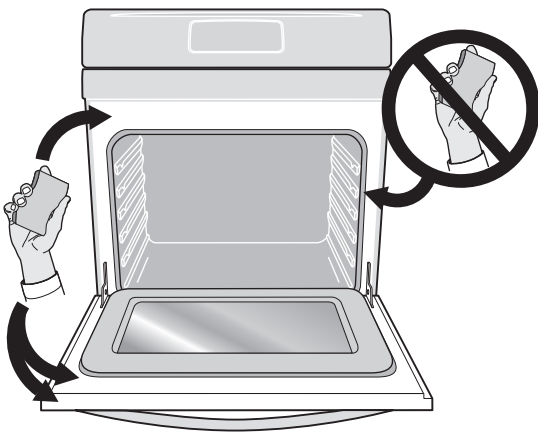
Figure 21: Clean around the oven door gasket
