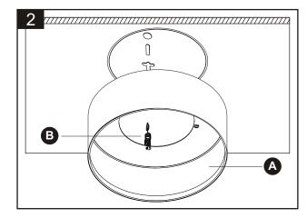
3. Attach spring hook (B) to holes in recessed fixture.
