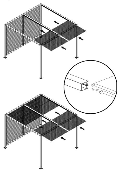
Slide two roof panels into the upper roof rails . Slide the other roof panels into the lower roof rails.
