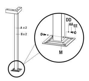
Attach one post base (M) to the bottom of each corner post (A)/(B) with washers (DD) and bolts (AA) using hex wrench (FF). Do not cover bolt caps in each step until at the end of step 10 when all bolt are firmly secured.
