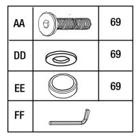
Attach slat (I) onto the three supports tubes (H) with washers (DD) and bolts (AA) using hex wrench (FF).
