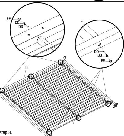
Inset the slat panel from step 4 into the frame from step 3.
