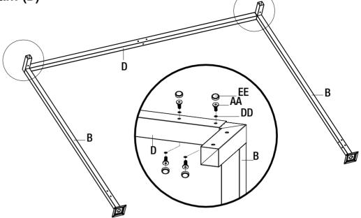
Attach the top of one corner post (B) to each end of cross beam (D) with washers (DD) and bolts (AA) using hex wrench (FF).
