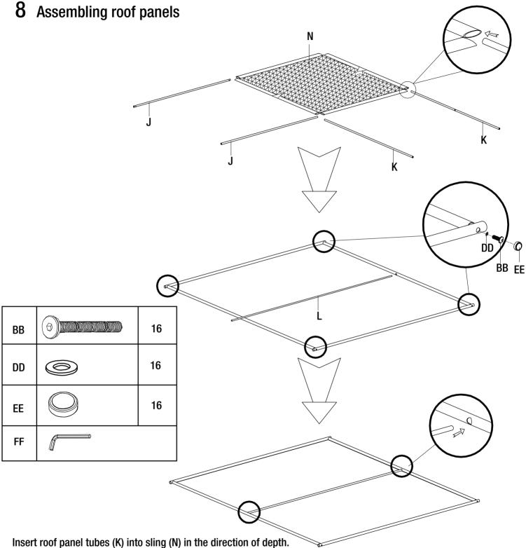
Insert roof panel tubes (J) into sling (N) in the direction of width.
