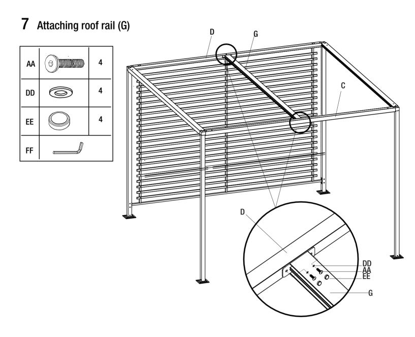
Attach the roof rail (G) to cross beam (C) and (D) with washers (DD) and bolts (AA) using hex wrench (FF).
