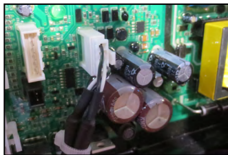
Figure 36 - Cable Wired to Board
