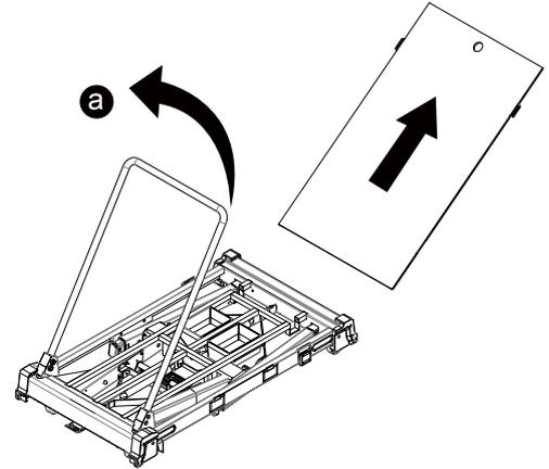
b. Turn over the panel to anti-slip work surface. Slip the panel into the corner protectors fasten the latches.
