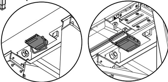
Make sure the lock is locked on.
