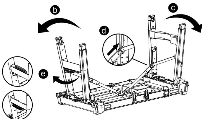
**NOTE:** You must open the narrower set of legs first, then the wider set of legs. Otherwise the legs can not open.
