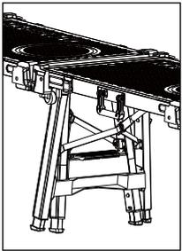
Put two Durabenches side by side, the narrower set of legs into the wider set of legs. A latch under the side of power strip can lock two Durabenches together.
