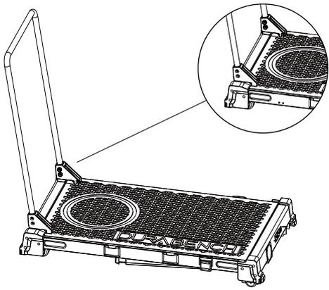
**NOTE:** Before using this product in cart mode, make sure that the handle are firmly locked in position and latches are closed tightly over the top panel.
