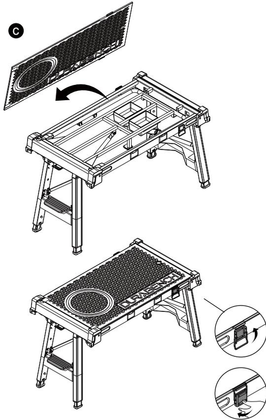
d. Turn the product over so the wheels are on the floor, open the latches, remove the panel and turn it over to the smooth surface, then fasten the latches.
