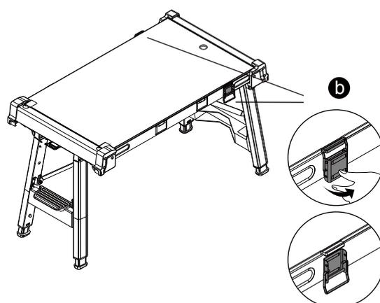
c. Remove the panel, turn it over so that the anti-slip work surface is face up, and place it back onto the scaffold. Fasten the two latches.
