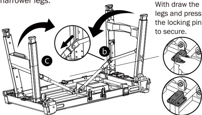
**NOTE:** You must close the wider set of legs first, then the narrower set of legs. Otherwise the legs will not close properly.
