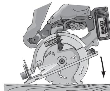
2. Tilt the saw forward and rest front of the shoe on material to be cut.
