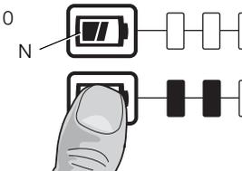
**NOTE:** The fuel gauge is only an indication of the charge left on the battery pack. It does not indicate tool functionality and is subject to variation based on product components, temperature and end-user application.
