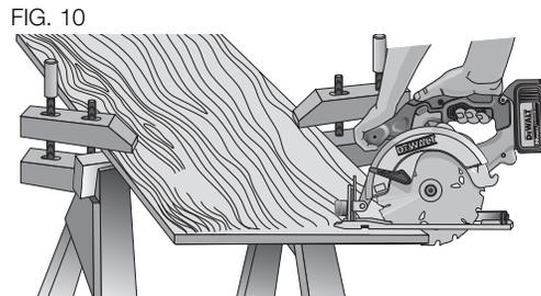
Figure 10 shows proper sawing position. Note that hands are kept away from cutting area. **To avoid kickback**, DO support board or panel NEAR the cut (Fig. 11). DON'T support board or panel AWAY from the cut (Fig. 12).
