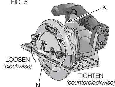
2. Remove the blade clamping screw (H) and outer clamp washer (P) only. Remove old blade.
