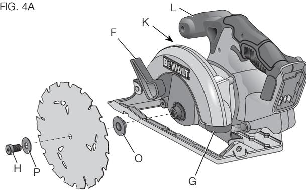
3. Place outer clamp washer (P) on saw spindle with the large flat surface against the blade with beveled side facing out.
