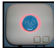
Solid red logo illumination indicates an power issue or no coil detected, blinking red indicates water leak
