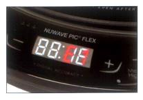
An E1 reading typically means that your PIC Flex does not detect cookware on its surface. This can occur for one of two reasons.
