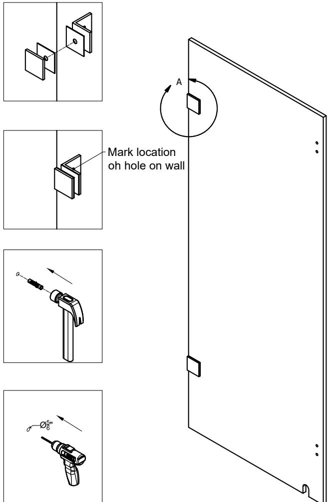
1. Affix the Wall Brackets (01) onto the Stationary Glass (02).
