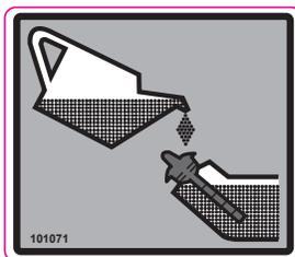
3. Add engine oil to the upper level of the oil filler hole. SAE 10/30 motor oil is recommended for most environmental conditions. The oil capacity is 1.16 quarts (1.1L).
