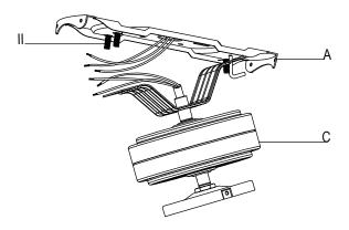
Once wiring is completed, lift the motor bracket on the top of the fan-motor assembly (C) so that the threaded studs (II) on the mounting plate (A) protrude through the slot in the motor bracket. Securely tighten the three locknuts (BB) onto the threaded studs (II), then try to shake the fan-motor assembly (C) to ensure that the assembly is tight.
