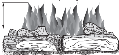
Figure 27 - Incorrect Burner Flame Pattern
