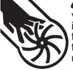
**⚠ WARNING:** Stop the engine before opening the vacuum inlet door. The engine must be stopped and the impeller blades no longer turning to avoid serious injury from the rotating blades. Gently tilt the handle of the screwdriver toward the back of the unit to release the latch while pulling up on the vacuum inlet cover with your other hand.
