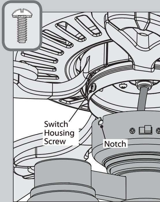
Partially install two of the switch housing screws found in the
