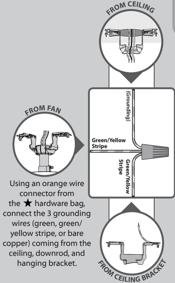
Using an orange wire connector from the ★ hardware bag, connect the 3 grounding wires (green, green/yellow stripe, or bare copper) coming from the ceiling, downrod, and hanging bracket.
