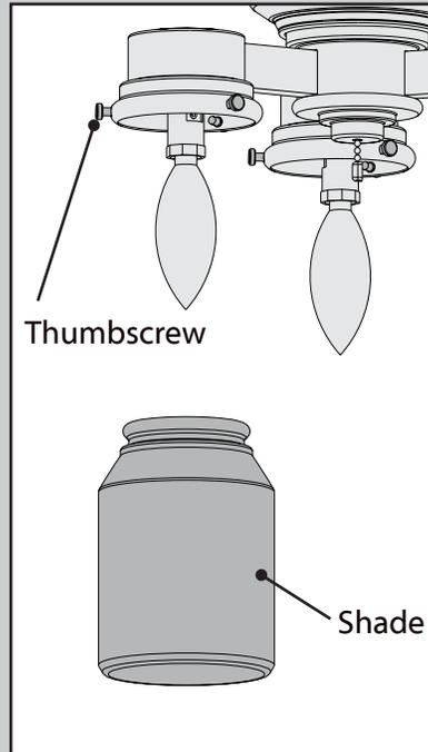
To install each shade, first loosen the thumbscrews. Carefully raise the shade to the light fixture and tighten all thumbscrews securely.
