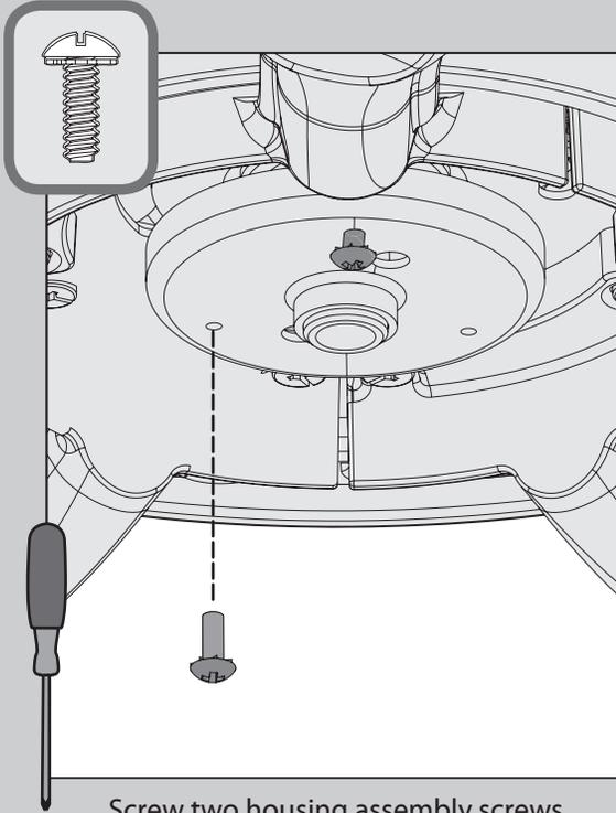
⊗ Screw two housing assembly screws from the ≡ hardware bag halfway into the motor housing. It does not matter which two screw holes you choose.
