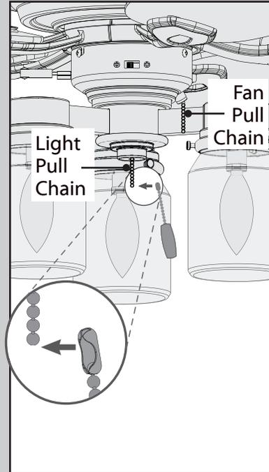
Connect the appropriate pull chain pendant to each of the short chains coming from the switch housing.
