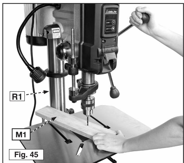
the spindle adapter and chuck fall from the quill.
