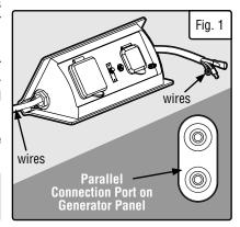
NOTE: The maximum voltage you can pull from the 14-50R outlet is 120V, you cannot pull 240V from it.
