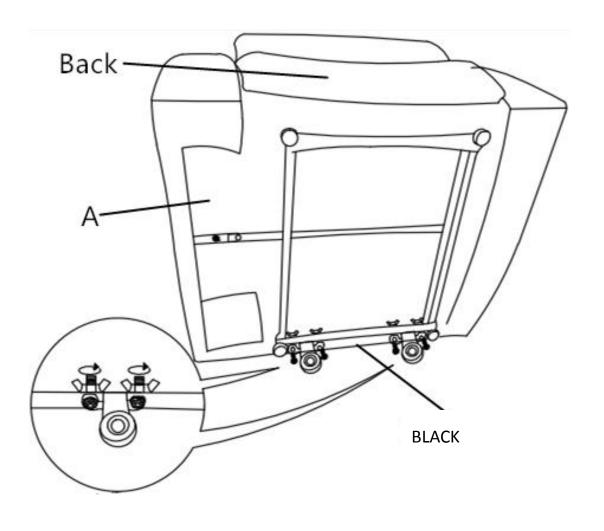
Attach backrest (B) to main frame (A) by aligning the metal grooves on backrest to brackets on the main frame as shown.
