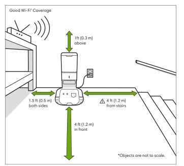
WARNING: To prevent the risk of your robot falling downstairs, ensure that the dirt disposal is placed at least 4 feet (1.2 meters) away from stairs.
