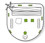
Important: Do not spray cleaning solution or water onto the sensors or sensor openings.
