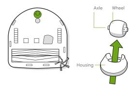
Important: A rear wheel clogged with hair and debris could result in damage to your floor. If the wheel is not spinning freely after you have cleaned it, please contact Customer Care.
