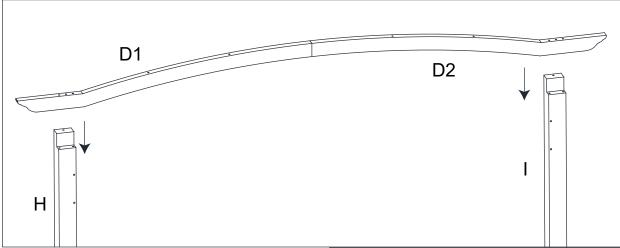
Attach rear beam (D1/D2) to post 1 (H) and post 2 (I). Secure with plastic washers (DD) and M6\*95 mm bolts (BB).
