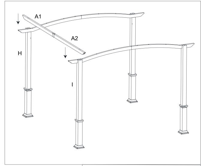
Attach left rafter (A1/A2) to the top of the beam and post assembly.
