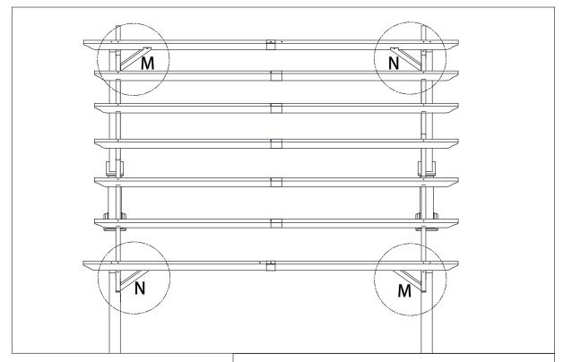
Attach a brace (N/M) to the pergola assembly as shown. Secure with washers (EE) and M6\*15 mm bolts (AA).
