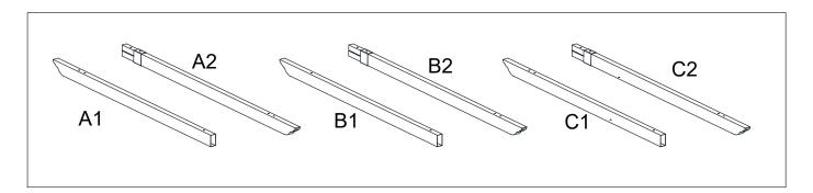
Set aside all rafter pieces. Assemble the left rafter by inserting the left rafter, male (A1) into the left rafter, female (A2). Secure the top of the joined rafter with a plastic washer (DD) and M6\*15 mm bolt (AA).
