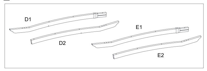
□ Set aside all beam. Assemble the rear beam by inserting the rear beam, male (D1) into the rear beam, female (D2). Secure the of the joined beam with a plastic washer (DD) and M6\*15 mm bolt (AA). Secure the bottom of the beam with a washer (EE) an M6\*15 mm bolt (AA).
