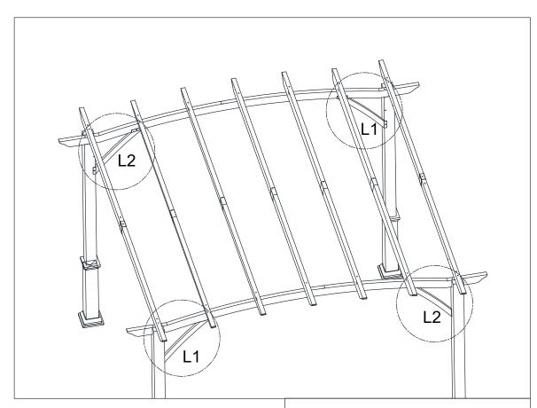
Attach a brace (L1/L2) to the pergola assembly as shown. Secure with washers (EE) and M6\*15 mm bolt (AA).
