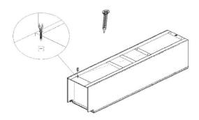
**Step 8**Secure the toe kick into the bottom of the cabinet (using two small screws(I) in each of the two clips).
