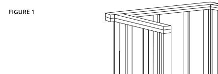
Box out for sub floor 6" x 6" core minimum size required
