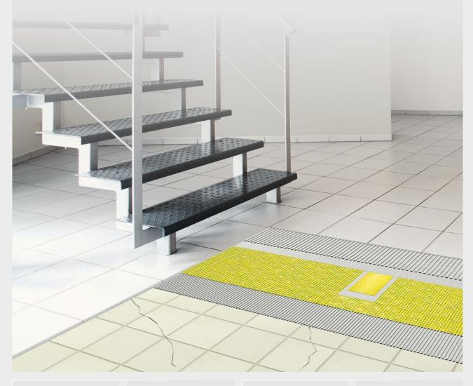
With its triple-layer construction, the multifunctional DURA-BASE CI++ matting system offers so much more than simply decoupling. The crack-bridging properties of the mat and its optimised shear force protection enable new tiles to be laid on old and damaged tiled floors, provided that these are still load-bearing.
