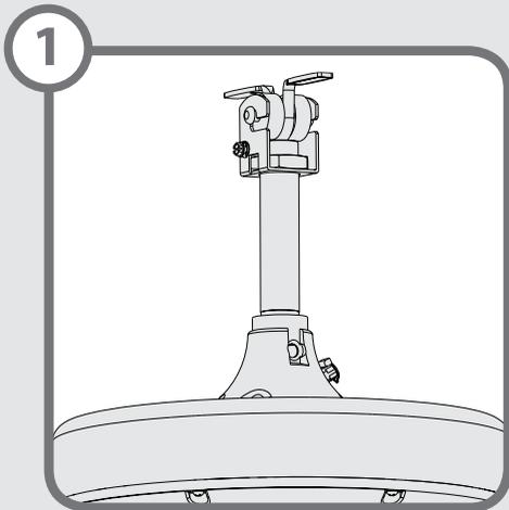
Install the fan according to the fan's manual, but do not install the canopy. Wire the grounding wire according to the fan manual's instructions.
