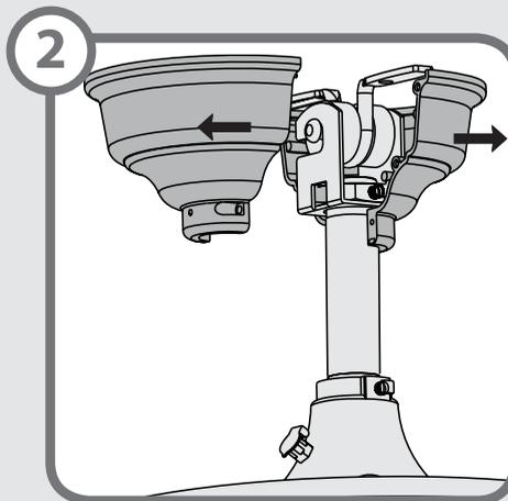
Remove the two canopy halves. With wiring exposed, it may be helpful to note existing wire connections or take a digital photo for reference. Remove the wire connectors that connect the wires from the outlet box to the fan, leaving the grounding wire connected.
