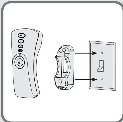
To install the transmitter cradle, remove the two screws holding your switch cover plate. Do not remove the cover plate. Orient the cradle by lining up the two mounting holes with those on the cover plate. Insert and tighten the screws. Do not over tighten.
