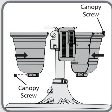
Push the two canopy halves from the kit together around the hanging system. Make sure that the receiver is tucked inside. Partially install the canopy screws from the kit into the screw holes. Slide the canopy up close to the ceiling. Tighten all four screws.
