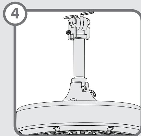
Reinstall the fan according to the installation manual included with the fan, but do not install the ceiling plate, canopy, or canopy insert. Rewire the grounding wire according to the fan manual.
