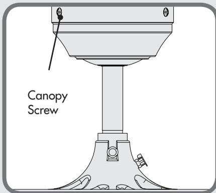
If your fan is already installed and the canopy is held by three screws near the ceiling as shown, follow **TYPE-C ASSEMBLY INSTRUCTIONS** on page 5.
