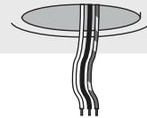
**CONNECT WIRES FROM RECEIVER TO WIRES FROM OUTLET BOX** - Using an orange wire connector connect the black wire (ungrounded) from the ceiling to the black wire from the receiver (marked "live in"). Connect the white wire (grounded) from the ceiling to the white wire from the receiver (marked "neutral in").
