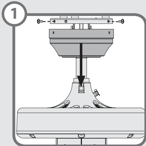
Remove the three canopy screws. Lower the canopy and the canopy insert. With wiring exposed, it may be helpful to note existing wire connections or take a digital photo for reference. Remove the wire connectors that connect the wires from the outlet box to the fan. Unhook the fan from the ceiling.
