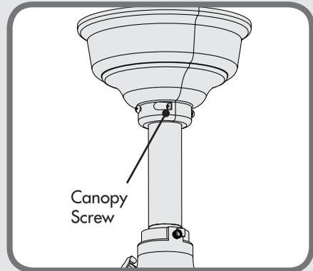
If your fan is already installed and the canopy is held by two screws near the downrod as shown, follow the **TYPE-B ASSEMBLY INSTRUCTIONS** on page 4.
