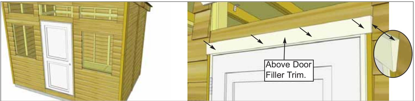
**88.** Before trimming door out, open/close door and confirm for level. Make any adjustments now. Locate **4AF - Above Door Filler Trim - Bevel**. Position over door casing with thick end of piece up and recessed slightly. Attach with **4 - 1 1/2" Finishing Nails**.
