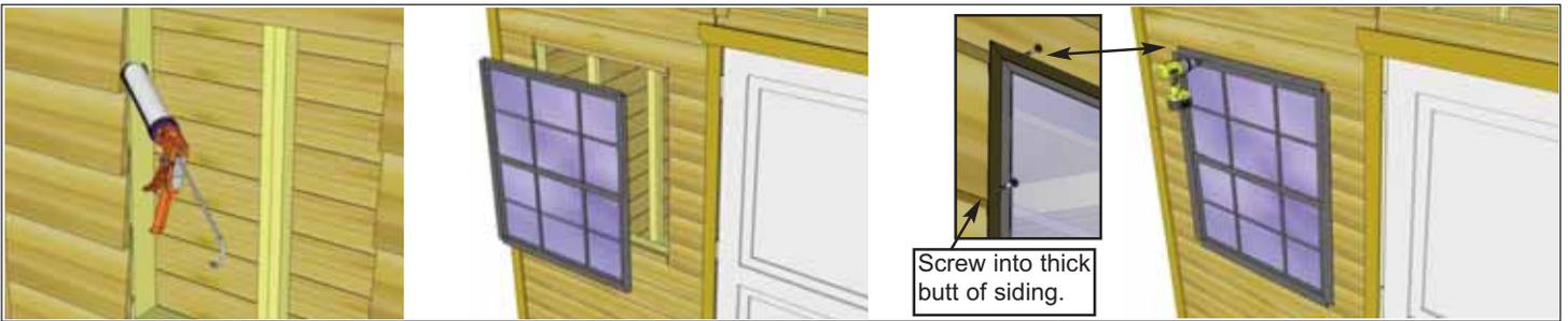
**90.** To reduce possible water from penetrating into the window cavity, caulk gap on both sides of window opening prior to installing the **4AI - Large Window Inserts**. Position insert in cavity and secure with **8 - 1 1/4" Screws**. Make sure to screw insert into the thick butt of the siding only.
