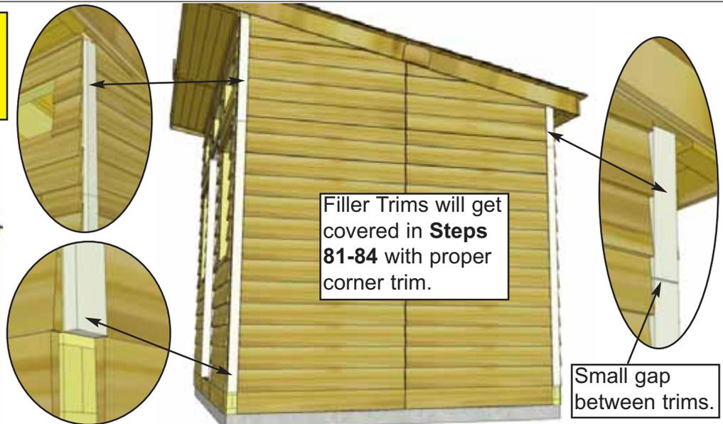
**80.** Position **4R - Filler Trim** (they serve as nailing strips) in corner of side wall, aligned flush with top of bottom skirting. Attach with **4 - 1 1/4" Screws** and repeat for all 4 corners. Next, attach **4S & 4T - Front/Rear Top Filler Trim** with **2 - 1 1/4" Screws** per piece.
