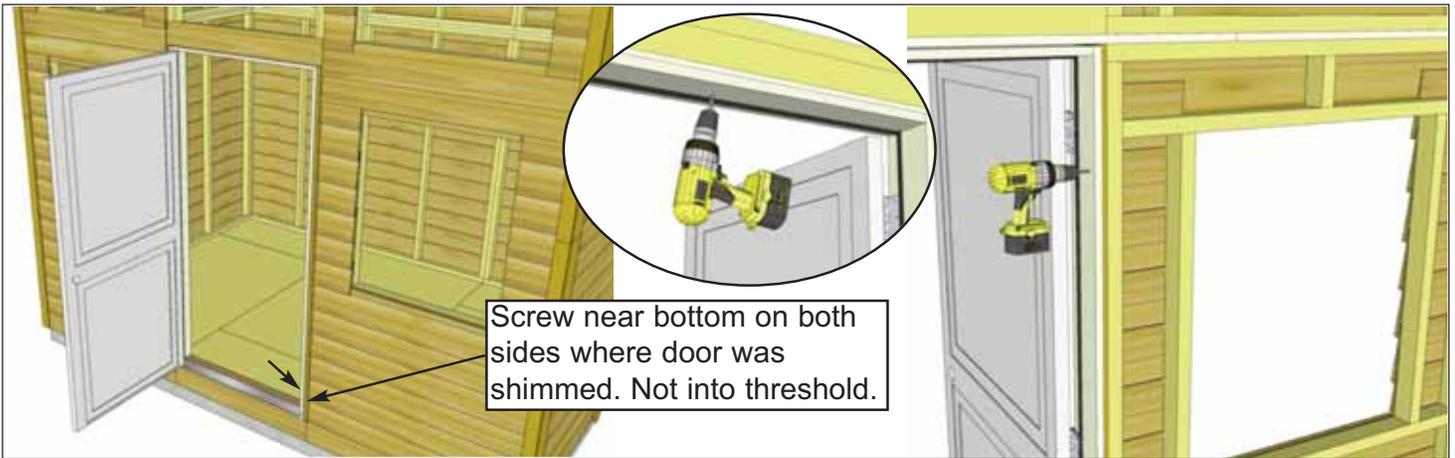
**87.** With door leveled in opening, open door and secure casing to shed framing where you shimmed. Use **2 - 2 1/2" Screws** on top and **3 - 2 1/2" Screws** on each side. Do not screw into threshold.
