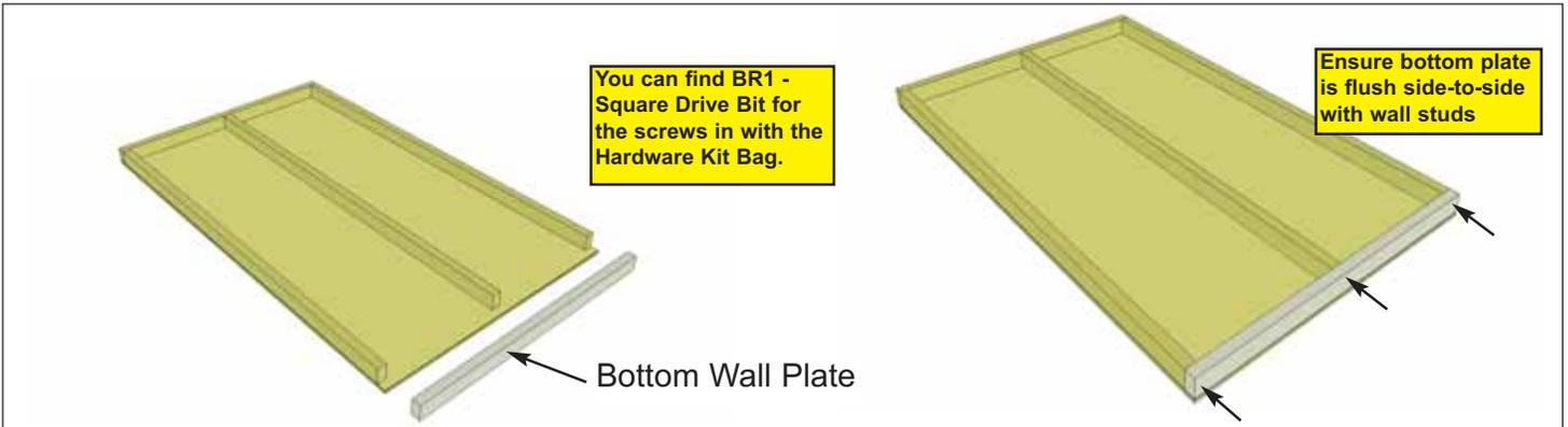
**14.** Carefully lay **2B - Solid Wall Panels** face down. Position and attach **2C - Bottom Wall Plates** to bottom of wall studs of each wall panel with **3 - 2 1/2" Screws**. Position so plates are flush with framing.
