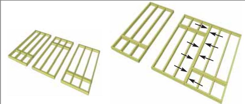
**5.** Complete all large and small frame attachments. Screw each completed section together with **8 - 2 1/2" screws**.
