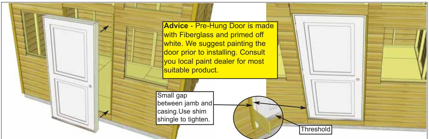
**86.** Locate **4AE - Pre-Hung Door**. Door opening is 38" w x 80 1/4" h. Place door in opening. Use **4AO - Shim Shingles** to shim door tight in cavity. Once shim is wedged in, cut excess shingle wood off. Insert 4-8 shim shingles.
