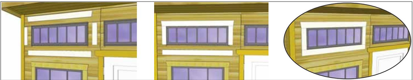
**95.** Position **4AL - Transom Window Trim** around window, doing a dry run first. Attach with as per **Step 94** with **4 - 1 1/2" Finishing Nails** per large piece and **2 - 1 1/2" Finishing Nails** per short piece. Complete other side window.
