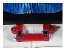
If bObi's dustbin is not fully engaged, her motor may not make proper contact with the battery's electrodes. If bObi does not restart her normal work after reinstalling her bin, or if she shows error 5 and her vacuum motor is not turning on, remove her dustbin, check that the connecting prongs on bObi are not stuck and can spring freely, then replace the dustbin securely.
