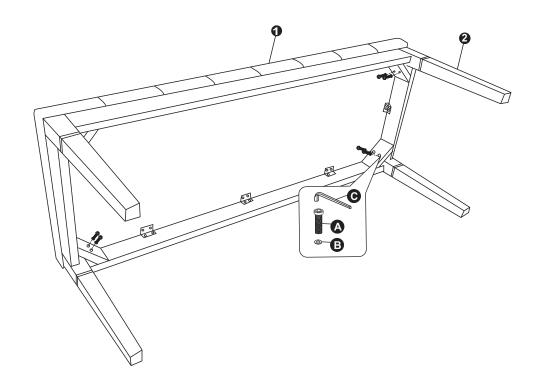
Attach Legs (2) to Seat (1) with Allen Key Screws (A) and eight Washers (B) into pre-drilled holes.
