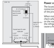
Installation space for water supply pipe
