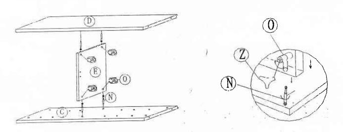
3.) Assemble Top panel (F) and Bottom panel (A). Use Cam-tool (Z) to tighten Cam-bolts (N) into Top panel (F) and bottom panel (A) and left/right side panel (C/D) Use Cam-tool (Z) to tighten Cam-locks (O) clockwise into the large holes of Left/right side panel (C, D). (See right picture)
