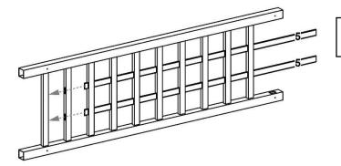
Insert vertical slats (part 5) through center cross rails and into bottom cross rail.
