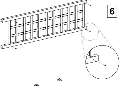
Using 1¼" screws, screw together trellis. Be sure that all parts are fully inserted into posts before securing.
