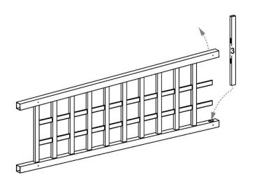
Separate top of post just enough to insert remaining top/bottom rail (part 3).
