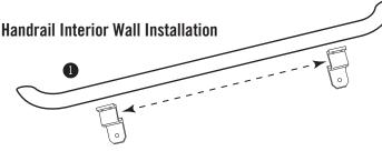
1. On the ground, layout handrail and wall brackets to ensure you will achieve your desired look and symmetry once the handrail is installed.
