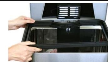
2) Remove the retainer ring from the can
