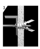
3.Tighten screw until flush with item.
