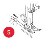
Pull both threads back and under the presser foot.
