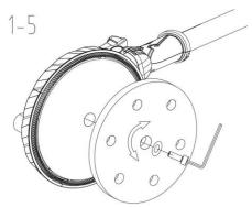
Attention: Only install the specified sanding pad on the machine.
