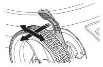
· The adjuster lever is spring loaded.
