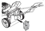
2 Lift the back shield and place the grass catcher frame hooks onto the grass bag brackets.
