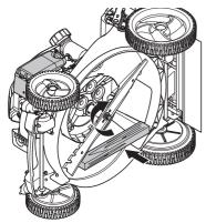
5 The bolt should be tightened with a torque of 35-40 ft. lbs./47-54 Nm. 6 Verify the spark plug wire is disconnected from the engine.
