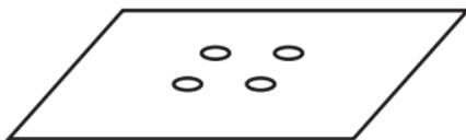
The plate inside is removable. Adding on screw is to prevent the plate moves inside but it is removable. If do not want to use the inside plate, take off the screw and remove the plate and use the black plastic screw to seal the hole or put the screw back.
