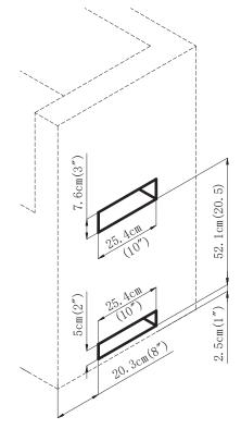
Proper ventilation is a required based on the above mentioned specifications for your grill to operate properly.
