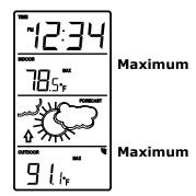
**Reset:** Hold the RESET button for 5 seconds to reset all minimum and maximum temperatures.
