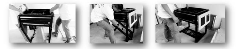
Grab the table base by the sides to lift up one side and screw in one wheel at a time. Screw in slowly to secure the wheels without damaging the treads on the base of the table.
