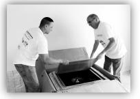
Removing the solid stainless steel grilling plate requires 2 adults due to its weight. Each adult should grab the handles located on each side and lift at the same time. Proper lifting procedures should be followed. Place solid stainless steel grilling surface to the side and away from box so as to have ample space to remove the actual base of the unit.
