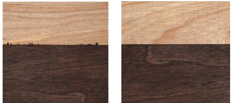
Apply a topcoat before stenciling to avoid the bleed seen on the left and keep a crisp, clean edge, as seen on the right
