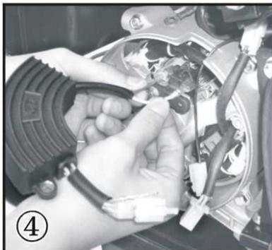
④ Remove the 2 wires of the AVR from the carbon brush.
