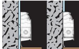
**Snap-on, hinged accessories** swing up for easy access to air vents and heating element or for removal of the front panel— even when wall material covers the accessory top. Precision piano hinges last for years.
