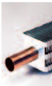
**5. High performance heating element. Maximum heat output. Fins won't loosen.** Double bent aluminum fins pack extra heating surface in a slimmer enclosure. Interlocking tongue-and-groove collars permanently bond fins to each other and to the tubing. Stops "pings and clicks". Tight bond assures maximum heat-transfer efficiency. End fins are of plated steel for extra ruggedness.
