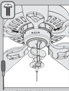
Install the third switch housing screw.
