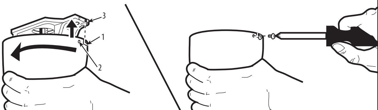
The canopy has two mating slots (1) and two mating holes (2). Position both slots on canopy directly under and in line with two screws in the mounting bracket (3). Lift the canopy, allowing the two screws to slide into the mating slots. Rotate the canopy until both screws from the mounting bracket drop into the slot recesses. Tighten screws securely. Install two screws into the mating holes of the canopy and tighten to secure the canopy to the mounting bracket.
