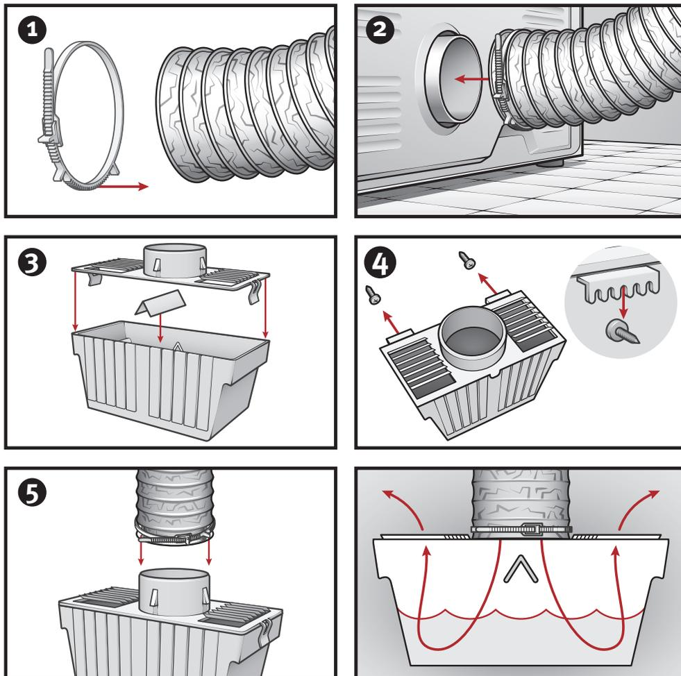
Note: Fill trap with water to 1" line indicated; replace lid. Replace lint filled water as needed. Because unit traps excessive moisture from dryer air, check water level on regular basis.
