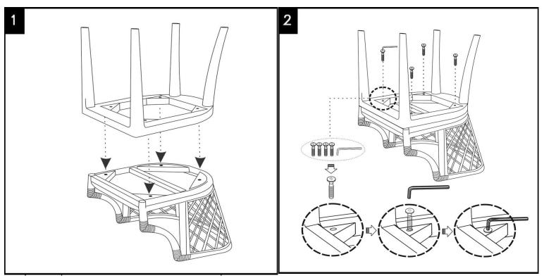
Assembly part A and B with Nuts and tighten with L key
